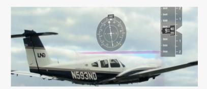
an alternative method of alerting the pilots for almost any condition ranging from nearby traffic conflicts, to proximity to terrain, or arrival an instrument approach minimums. It's similar to the concept of a highway rumble strip, intended to keep a driver in their lane.
